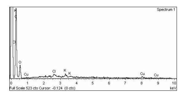
Fig. 3. The EDAX of the elytron without using gold as adhesive.
