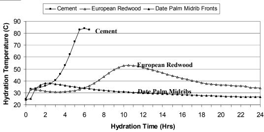
Fig. 1. Exothermic hydration curves of untreated date palm-cement and European redwood-cement mixtures without chemical additives comparing with net cement.
