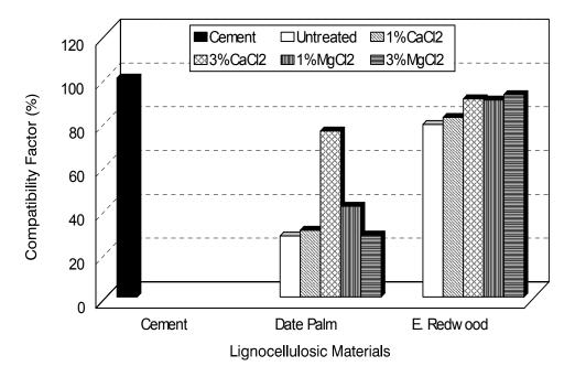
Fig. 4. Effects of chemical additives (CaCl<sub>2</sub> and MgCl<sub>2</sub>) on the compatibility factor of wood-cement mixtures as compared to cement and untreated wood-cement mixture (untreated).
