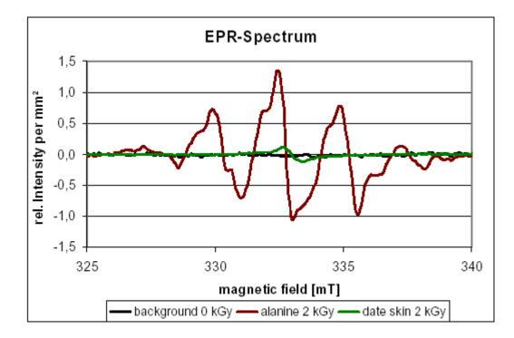
Fig 1. EPR-spectrum of date skin in comparison to alanine dosimeters.
