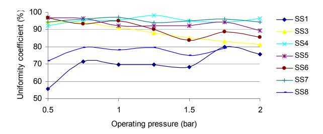
Fig. 4. Uniformity coefficient at various operating pressures for different pipes.
