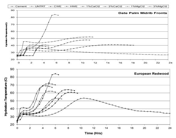
Fig. 2. Exothermic hydration curves of the mixtures of midribs date palm fronds and European redwood with cement under different treatments as compared to net cement. For legend see section of materials and methods.
