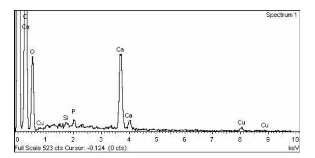
Fig. 4. The EDAX of the hind wing without using gold as adhesive.
