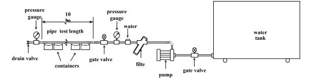
Fig. 1. Laboratory experiment layout.
