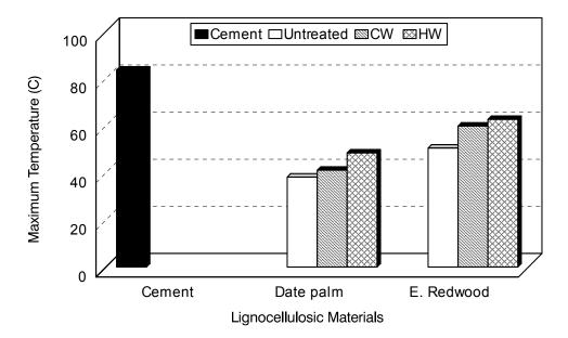
Fig. 3. Effects of cold water extraction (CW) and hot water extraction (HW) of date palm and European redwood on the maximum hydration temperature of wood-cement mixtures with comparing to cement and untreated wood-cement mixture (untreated).
