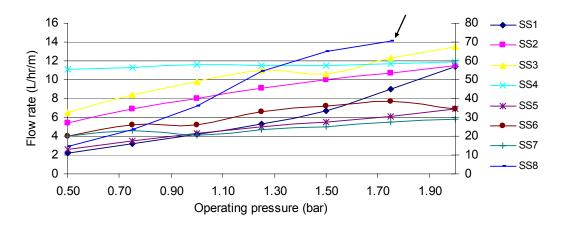
Fig. 3. Curves represent pressure and discharge for subsurface irrigation pipes (the vertical axis of right-special Curve specified arrow).
