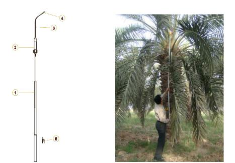
Fig. 1. Sketch of developed electrical pollinator (left) and the pollinator in work (right).
