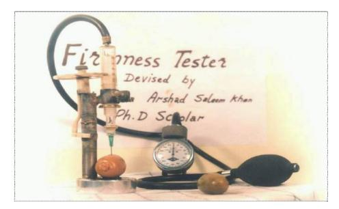
Fig. 1. Hardness testing device for 'Dhakki' dates developed by the author (Dr. Shahzada A. Saleem Khan).
